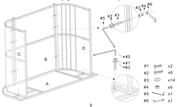
Step 3.Attach one shelf (part #E) to assembled parts (part #B,C&D) using short bolts (part #1), washers (part #3) and allen key (part #5).
