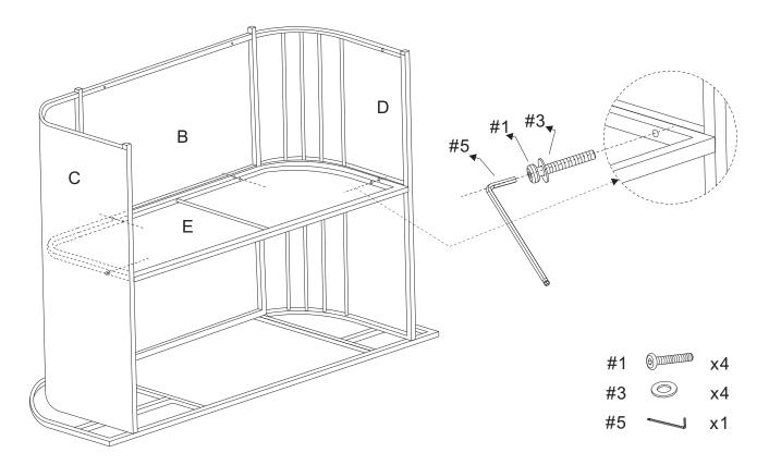
Step 4. Attach another shelf (part #E) to assembled parts (part #B,C&D) using short bolts (part #1), washers (part #3) and allen key (part #5).
